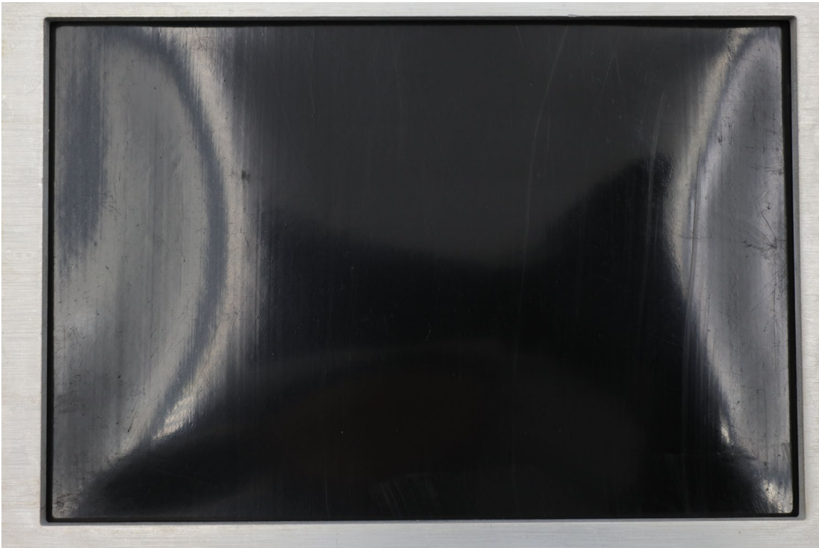
Figure 7. Sample 13204-1 specimen 1 after 2500 hours of exposure.
