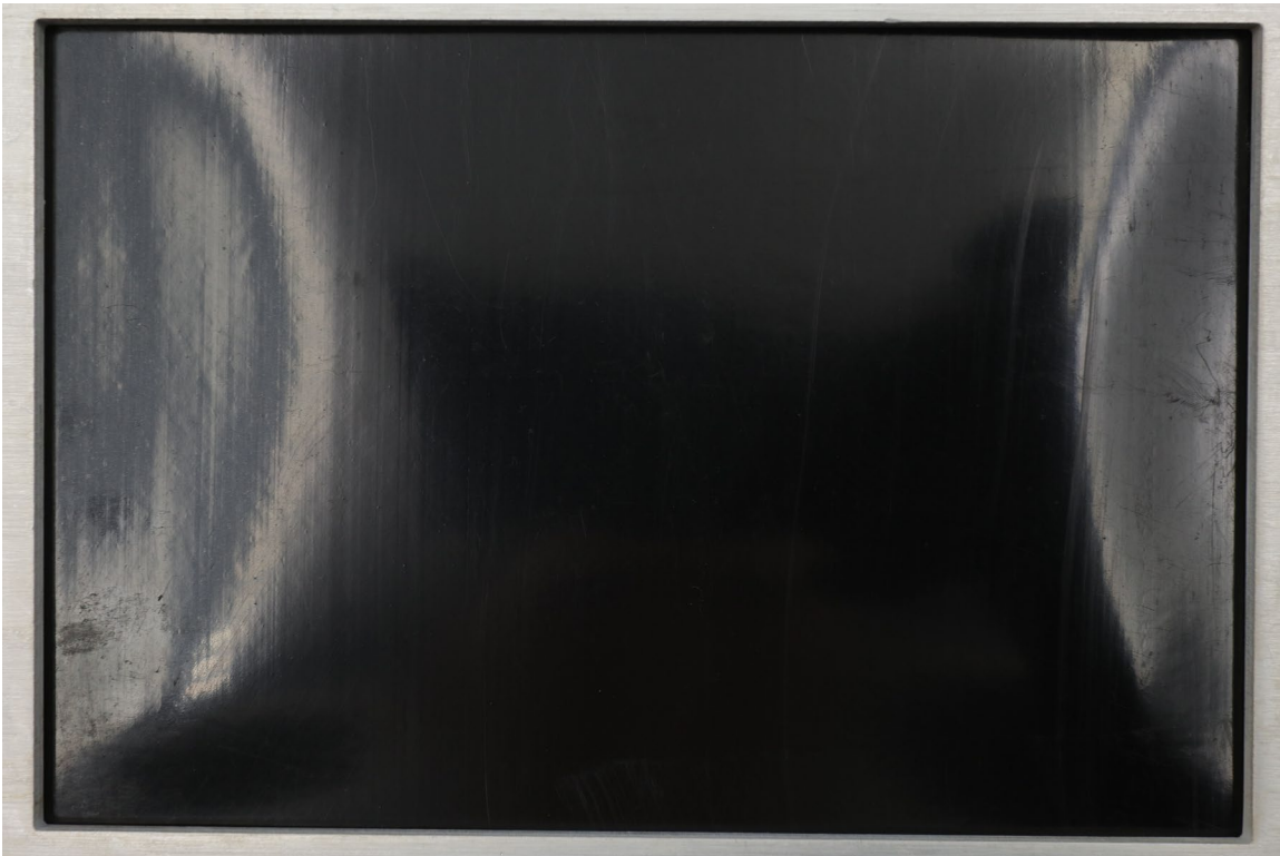
Figure 5. Sample 13204-1 specimen 1 after 1500 hours of exposure.
