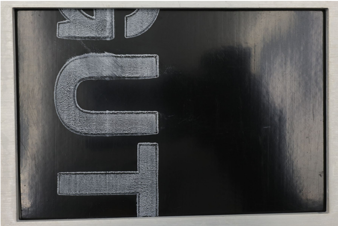
Figure 14. Sample 13204-1 specimen 2 after 2500 hours of exposure.
