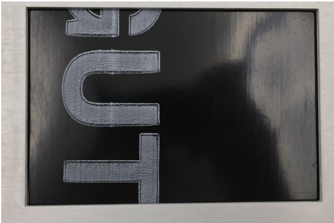
Figure 10. Sample 13204-1 specimen 2 after 500 hours of exposure.
