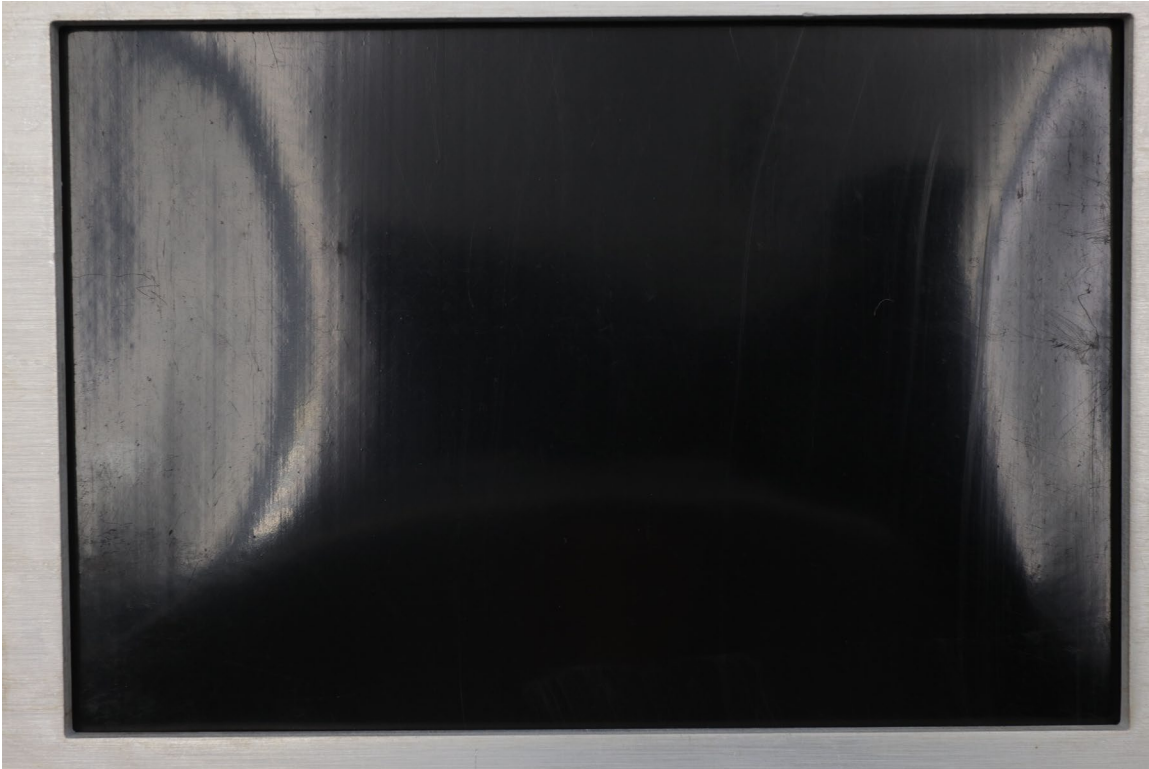
Figure 4. Sample 13204-1 specimen 1 after 1000 hours of exposure.
