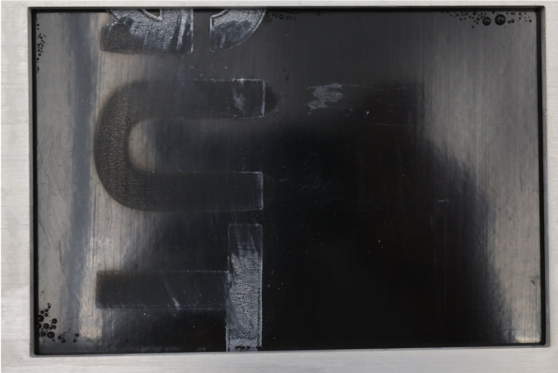
Figure 15. Sample 13204-1 specimen 2 after 3000 hours of exposure.
