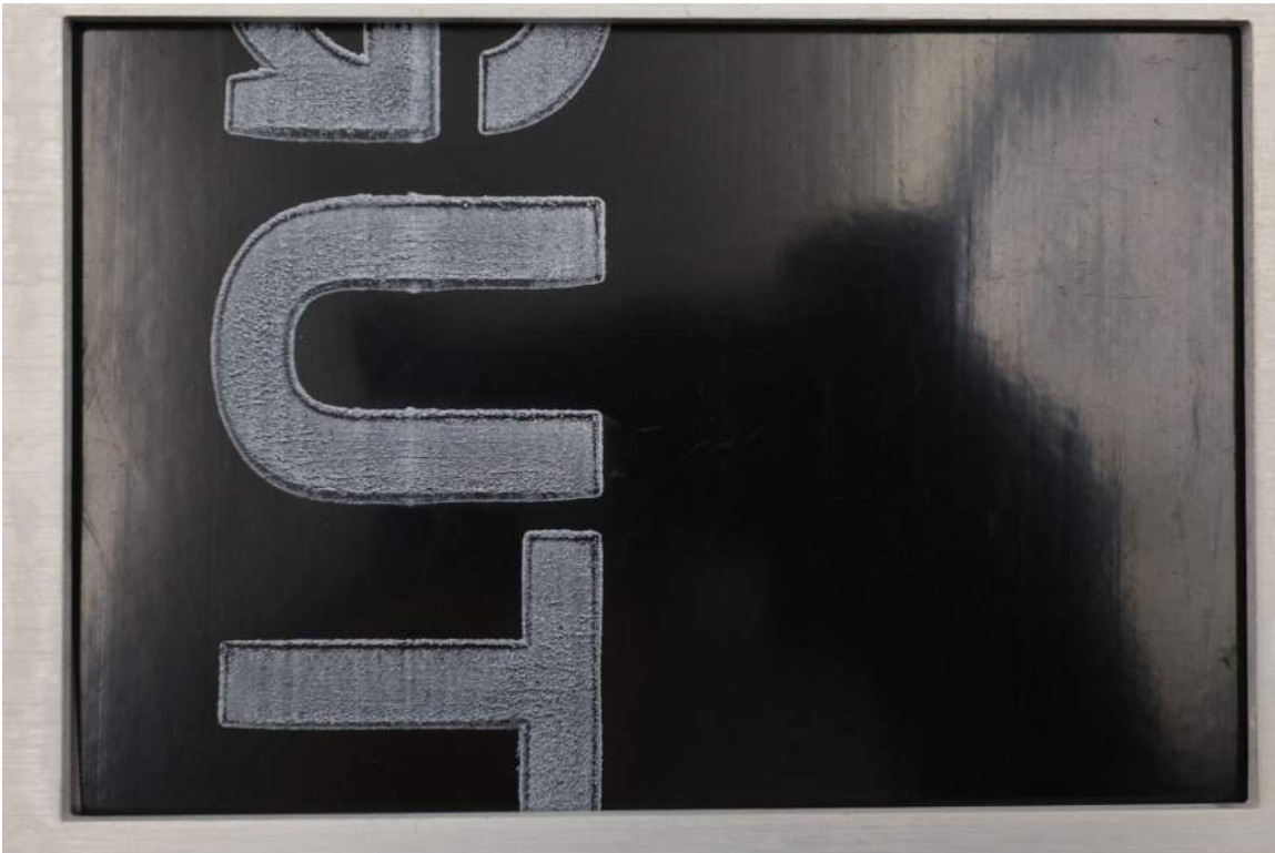
Figure 12. Sample 13204-1 specimen 2 after 1500 hours of exposure.
