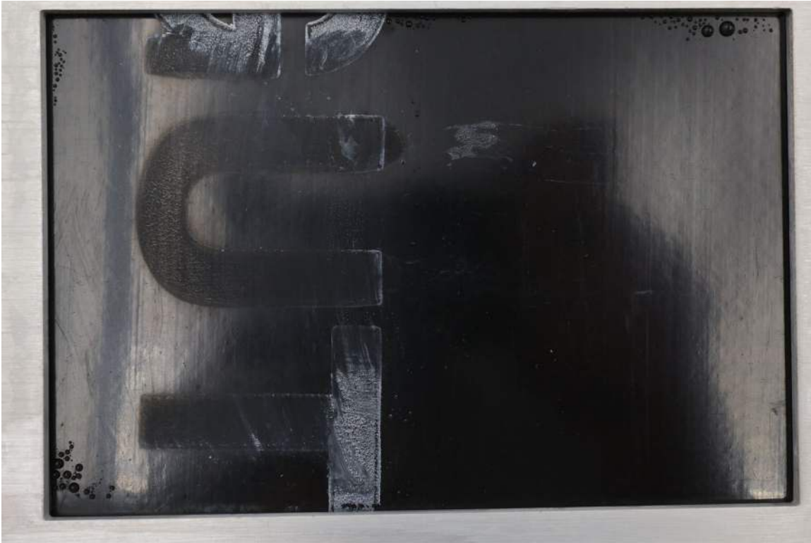
Figure 15. Sample 13204-1 specimen 2 after 3000 hours of exposure.
