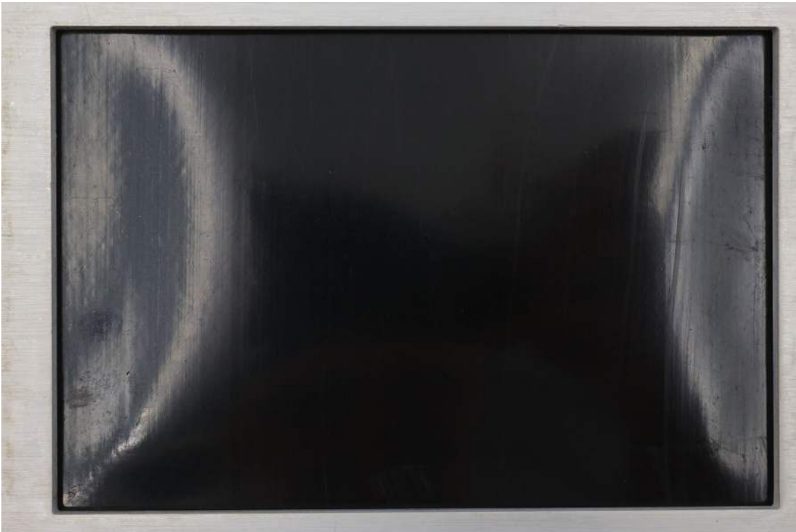
Figure 3. Sample 13204-1 specimen 1 after 500 hours of exposure.
